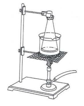
Watch the unknown liquid carefully. The liquid will begin to evaporate rapidly, and its volume will decrease. The amount of liquid placed in the flask is much *more* than will be necessary to fill the flask with vapor at the boiling water temperature. Excess vapor will be observed escaping through the pinhole made in the foil cover of the flask.
